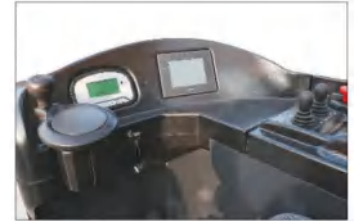
Camera and positioning: Optional positioning system offers easier pallet handling at height through camera system.
